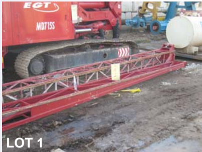
"EGT" MD-715 multi purpose drill rig, No. 1270 (2008) with 2 nos. extension booms (6m each) & boom attachment
