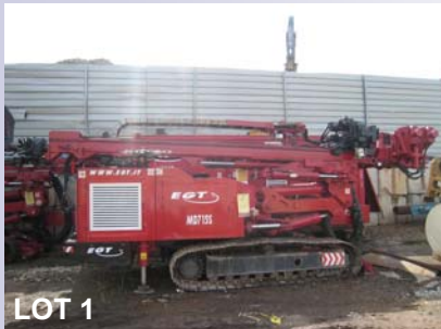
"EGT" MD-715 multi purpose drill rig, No. 1270 (2008) with 2 nos. extension booms (6m each) & boom attachment
